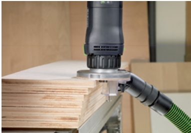
Chamfering plastic or solid wood veneer.
