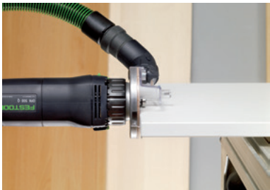
Rounding plastic or solid wood veneer.
